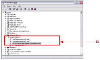
If the items (12) and (13) are present, the USB driver is installed correctly
